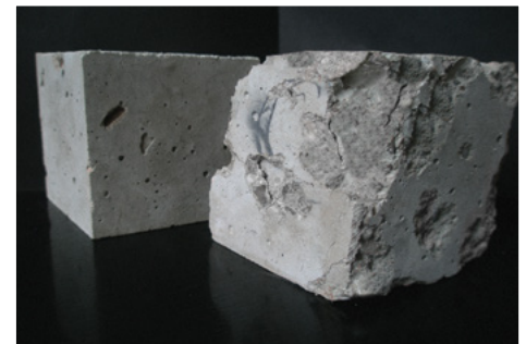
Test specimens after fire testing: specimen with and without fibres.
