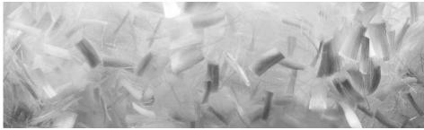
PP PE PLA PBS PBSA fibres 1.2 - 150 dtex | 13 - 145  $\mu$ m ø | 1.5 -> 20 mm
